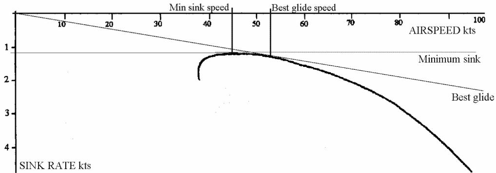
Also shown in the above graph is the minimum sinking speed, which is about 1.1 kts at 45kts airspeed
