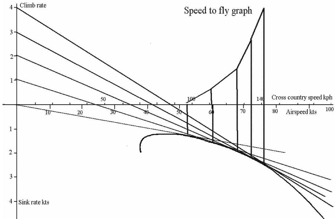
This graph was used by Paul McCreeady who placed this information onto a ring that neatly fits around the face of the vario. The device is of course known as the Mc Cready ring, and tells us the optimum speed to fly for any given sink.
