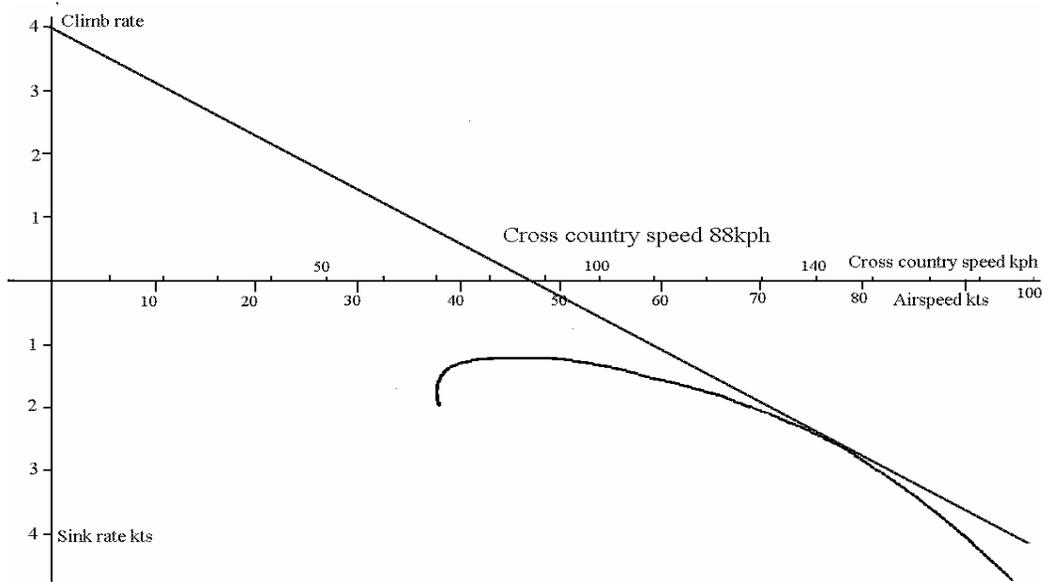
*This shows clearly that increasing climb rate is highly beneficial when maximum cross-country speed is required. In this case an increase in speed of over 11%. Even if the pilot used a conservative 2kt ring setting his cross-country speed would be 85kph.*
