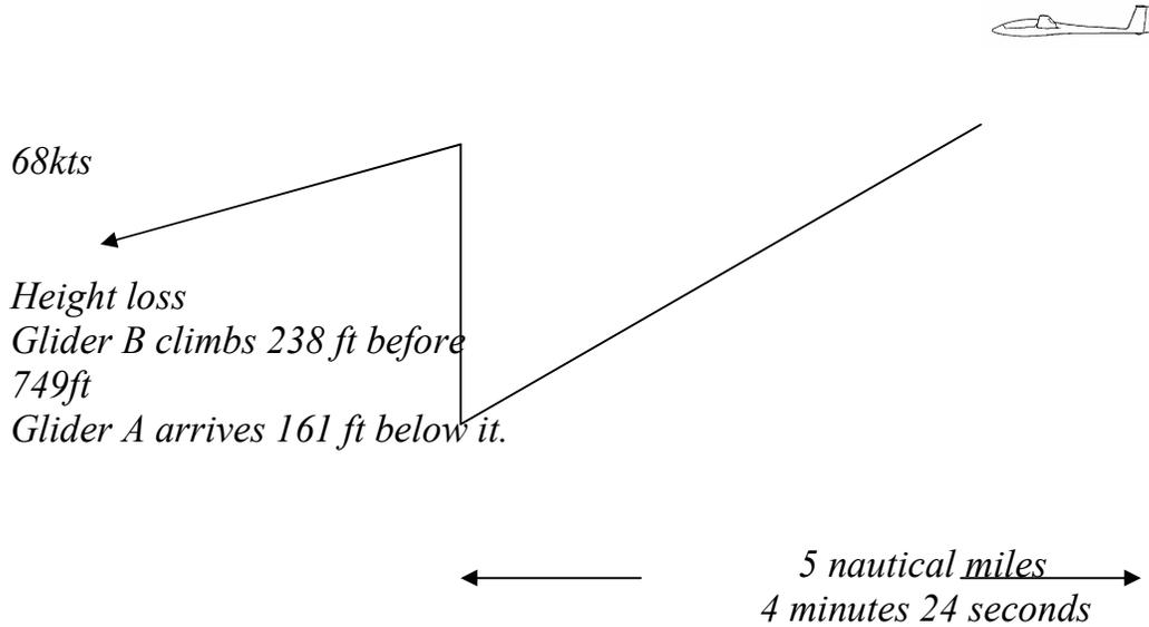
*In the last case it can be seen that the glider flying faster towards the thermal will reach it first, and start to climb in it. By the time the second glider arrives, it will not only have made up the extra height loss but also have gained a significant height advantage over the first. In this way the average cross-country speed will be increased. To find out exactly how fast a particular glider should fly in any set of conditions then reference should once again be made to the polar curve.*
