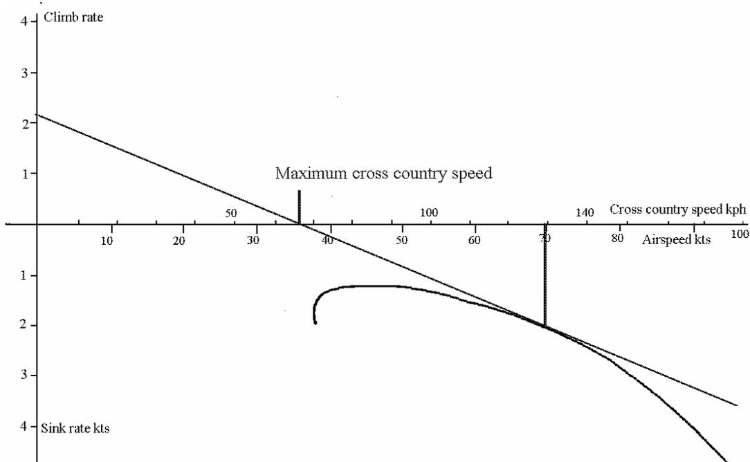
*In this diagram the climb rate is plotted on the positive Y-axis and a line drawn from this to a point where meets the polar tangentially. At the point it crosses the X-axis is shown the maximum theoretical cross-country speed; in this case it is 68 kph.*
