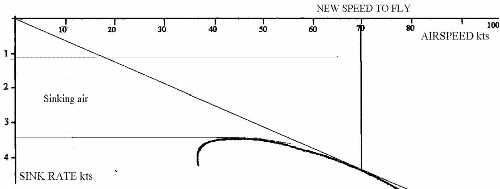
This polar shows a glider flying through air sinking at about 2.2kts; the new speed to fly for best glide is now 70kts. Moving the polar curve down the Y-axis 2.2kts has simulated the sinking air.
