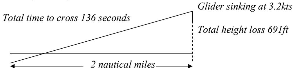
When looking at the two examples it can be seen that the glider flying faster than best glide loses less height than the other. This is because it is spending less time in the sinking air than the slower glider despite the fact that it is sinking faster by flying faster. Once again this principal of flying faster in sinking air for maximum distance can be shown on the polar curve and the cruising speed optimized for each set of conditions.
