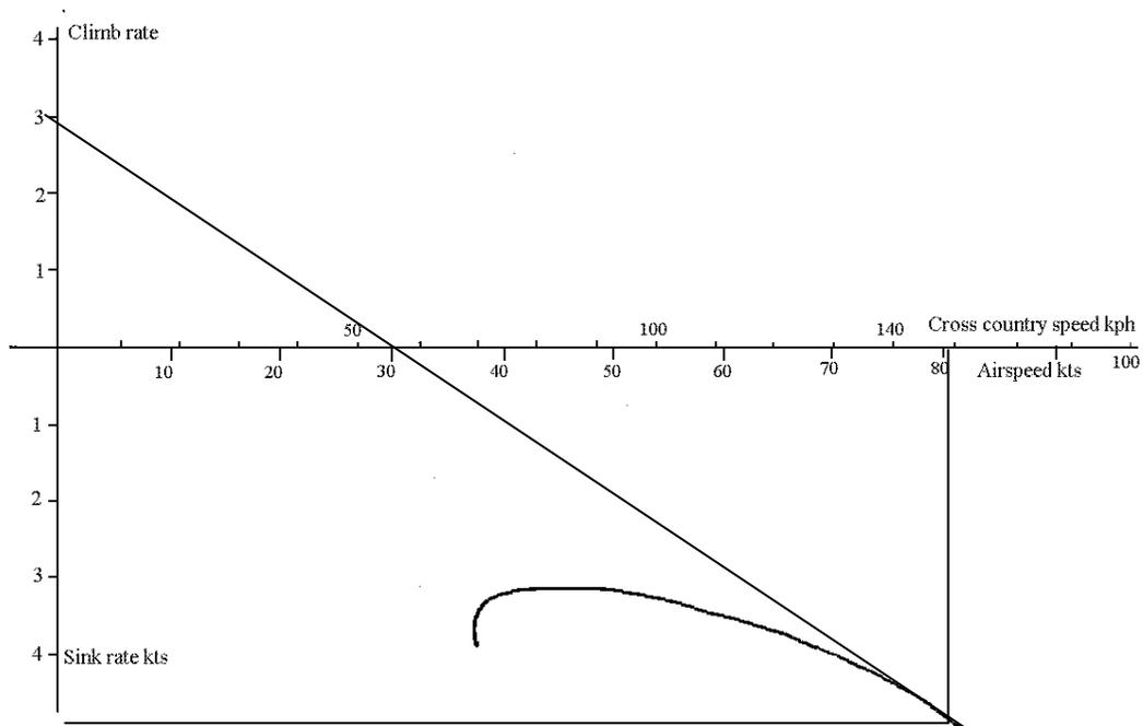
*As was demonstrated earlier Mc Cready theory demands a higher cruising speed when flying through sink, and if this is done then the glide angle will be optimized. In the above case not only is a higher speed demanded due to the sinking air mass but also due to the climb rate being set on 3kts.*
