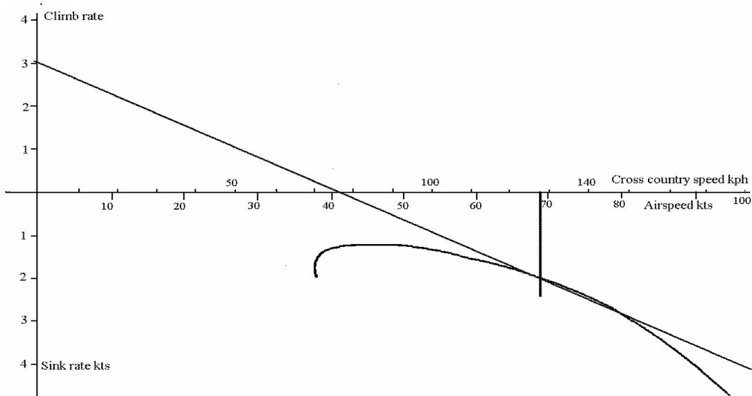
This now shows us that flying in conditions that produce 3kt thermals and still air glides, then using a 2kt ring setting will give us a cross country speed of approximately 76kph. This speed should now be compared with the pilot who flies with a ring setting of 3kt.
