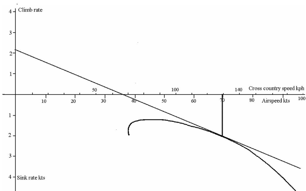
If all these points are plotted on the graph then we can form a new chart of correct speeds to fly for different sinking airmass conditions. For instance if the glider is flying in an airmass that is sinking at 3kt then the correct speed to fly would be 72kts.
