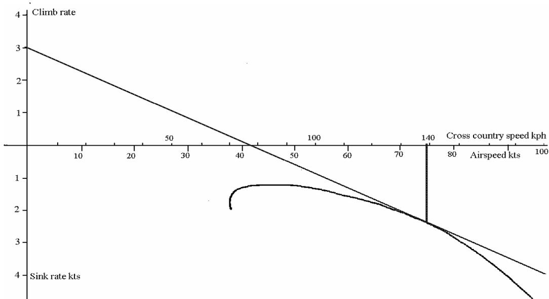
*It can be seen that this pilot will achieve a cross-country speed of about 78kph by flying at the correct Mc Cready speed for these conditions.this shows an improvement of 2kph or 2.6%.*
