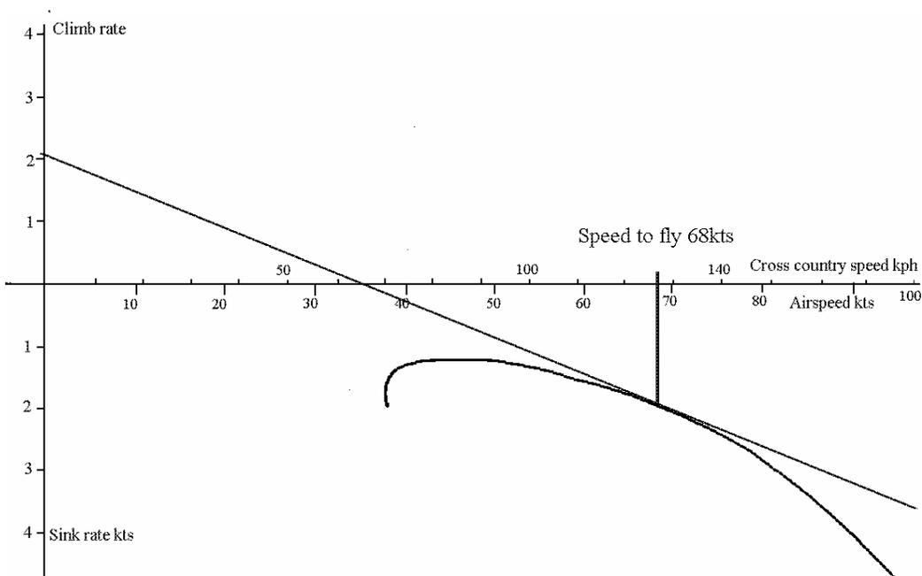
To find out what the cross country speed will be with this 2kt ring setting in 3kt conditions, then a new line should be drawn from 3kt on the positive y axis down to a point on the polar such that it crosses the polar at 68kt on the positive x axis.
