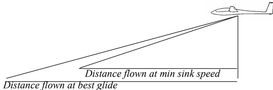
*however not by the same ratio and it is this maximum ratio of forward speed to sinking speed that gives the best glide ratio. Above is shown the total distance flown and height lost for a glider flown at its best glide speed and its minimum sinking speed for a given time period.*
