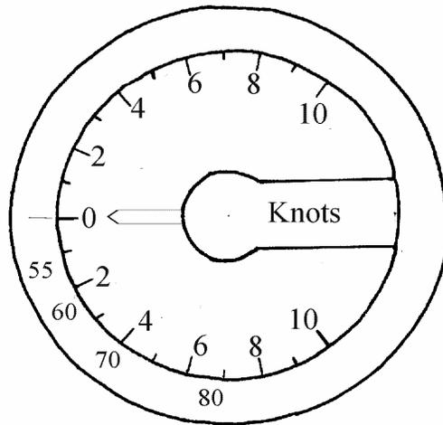
*If you have ever flown with a vario fitted with a McCready ring then you may have noticed that the ring is not fixed, but is free to rotate around the face of the dial. This is because the device has a second function, in that it will provide the optimum speed to fly if the next climb is known.*
